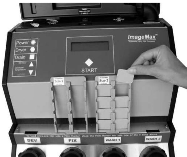
**TIP:** To load film, place the film holder lower tab (magnet) into one of the 4 slots over the holding tanks as shown. Then, load intra-oral films into the film holder with a light touch. Load the bottom first, then work up to the top.
